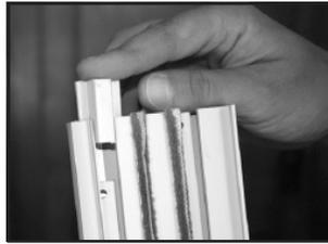
7. Snap the balances onto the clips by pressing on the outside edges of jambliner. Check to ensure that the "hooks" on the clip interlock with the edge "hooks" on the jambliner.
